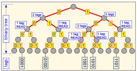
opposite bit become temporarily inactive waiting for the next traversal. When only one tag responds at any stage of the traversal, that tag can be read. Proceeding in this fashion over the whole ID string (if necessary), the reader must inevitably find all tags in the field if their ID's are unique and all the tags are able to follow the traversal.
