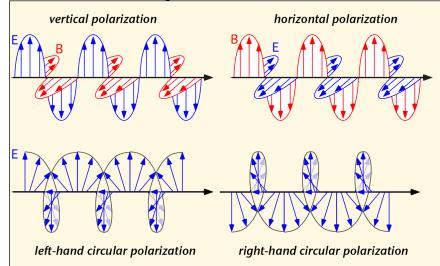
The best power transfer between antennas is obtained when their polarizations match. Thus the best read range is obtained from e.g. a vertically polarized reader antenna transmitting to a vertically
