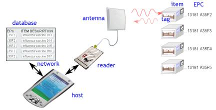
description below will assume their use. Variants are also available: *semi-active* tags incorporate a battery to power the integrated circuit, but still use reflected waves (*backscattering*) to communicate with the reader. *Active* tags incorporate both a battery and a radio transmitter, and are much more costly than passive tags, but also more versatile.
