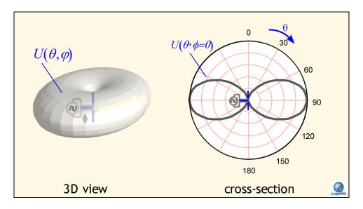
The MPR5000 integral antenna behaves like a dipole oriented parallel to the short edge of the card. Thus, radiation is mainly forward (looking along the long axis of the card), up, and down, but with very little power radiated to the left or right of the card. The radiation pattern can be regarded as a torus (doughnut) with axis along the short side of the card.
