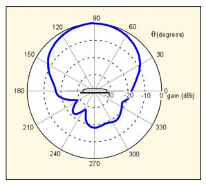
of this antenna along the azimuth (horizontal plane for a typical vertically-mounted antenna).
