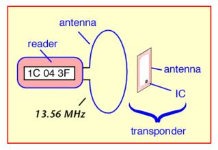
identification badges and credit cards with enhanced functionality. Typical read range varies from a few cm to a meter or so (a few inches to 3 feet), again dependent on reader antenna size.
