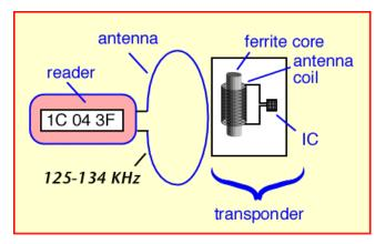
proximity to the reader antenna to be read; read ranges are comparable to the size of the reader antenna, typically a few 10's of cm (5-10 inches) for a small reader antenna. Because the induced voltage per coil winding is also very small at these frequencies, the tags are composed of many turns of wire, often
